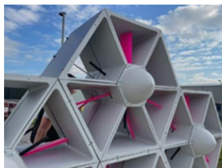
Figure 2: Katrick Technologies Building-Mounted Wind Turbine (image submitted in evidence by Mott MacDonald)
